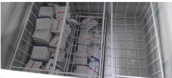
***DF without Ice Lining***, welcomes early frost formation, grill baskets with large windows, the cartons slip down to the bottom, ***get matted***, CCH may not remove till the stock gets over or while removing vials / ampoules may get broken incurring
