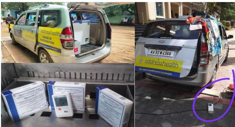
more than enough to reach the outreach session site. On reaching the session site, the ILDF through Voltage stabilizer connected to 3 pin power plug using extension cord so that the ILDF regains -25 °C from say -22 °C.
