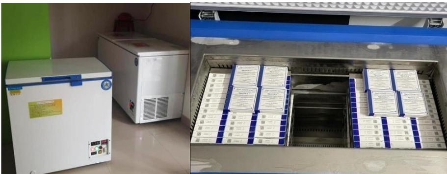
Frost free, toplid Ice Lined Deep Freezer [ILDF] with sliding trays, provides adequate free air circulation space maintained in Addresshealth, Bengaluru, Karnataka, India.
