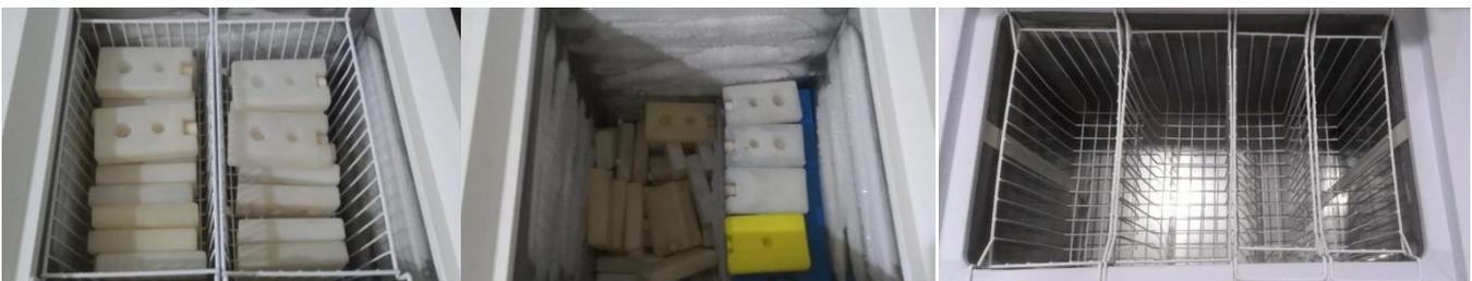
Above Deep Freezers in the public sector are not having Ice-Lining. Frost formation inside the DF is an unwelcome almost unavoidable phenomenon as long as ambient air has water vapor. **While defrosting, there is a threat of sacrificing vaccine either through breakage or through thawing or both.**
