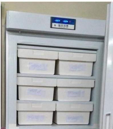
Deep Freezer with vertical door: cabinet temperature sharply rises even with short opening as heavy cool air from the cabinet space slips down and warm room air fills the cabinet resulting in Temperature Excursion with every opening like domestic refrigerator.
