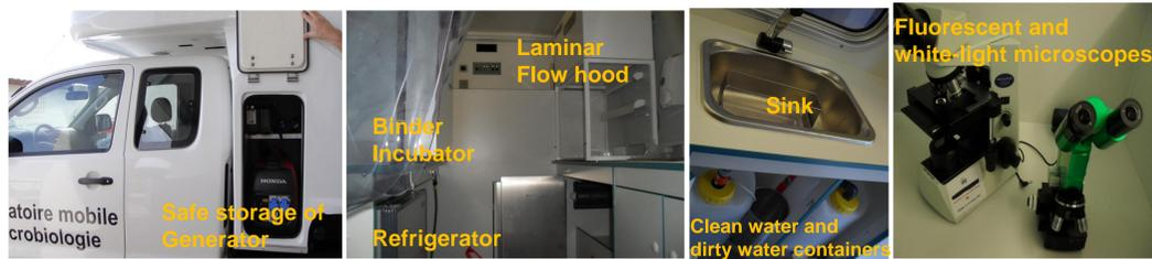
Figure 1: Interior view of LaboMobil® included tailored microbiological class2 laminar flow
