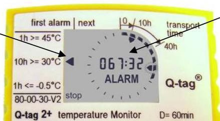
In this example, at 67 hours 32 minutes, the 30°C alarm was triggered for more than 10 hours.
