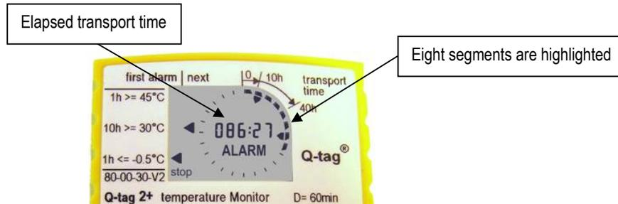
"OK" remains visible until any alarm is detected. It is then replaced by "ALARM" and more information is displayed.
