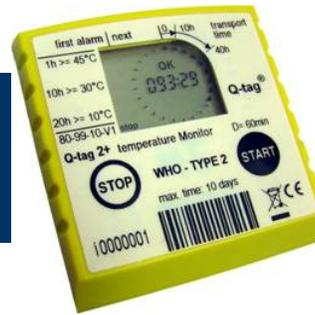
The figure below describes the Q-tag® 2 plus device (in the figure the screen is displayed in TEST mode to show all features).
