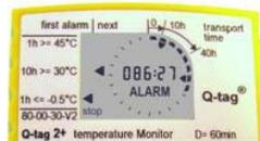
ALARM sign is seen in the middle of the screen. ◀ symbol indicating the type of alarm also appears on the left side of the screen pointing to the types of alarms. The ◀ symbol closest to the left edge indicates the first alarm, while all later alarms are indicated in the "next" column.
