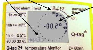
12. The temperature displayed in the LCD centre is the recorded minimum during the blinking time segment.
