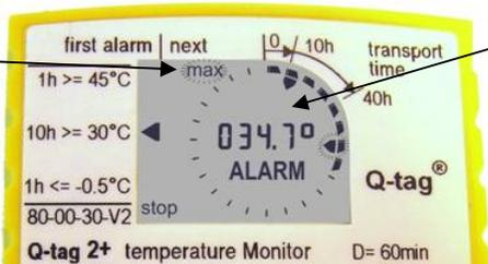
With the next push to the **START** button, the screen in the middle displays the highest (maximum) temperature recorded during the violation which was 34.7°C.
