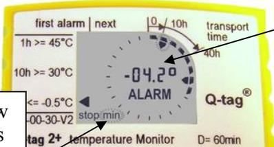
Since this alarm involves low temperatures, the **min** sign is flashing indicating that the temperature displayed is the minimum temperature recorded.
