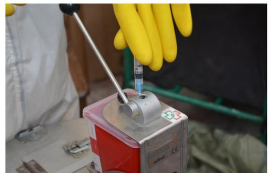
Figure 35. Mutilating syringes using manual needle cutter
