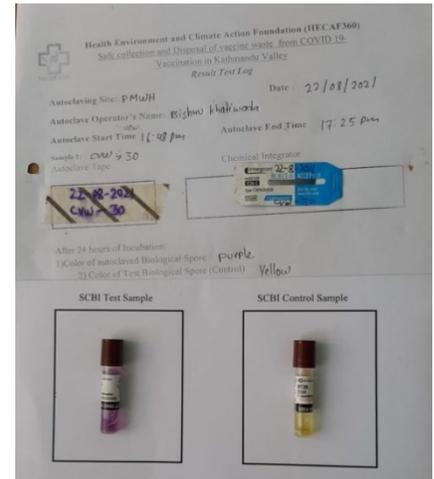
Figure 33. Autoclave test log with record of all testing indicators
