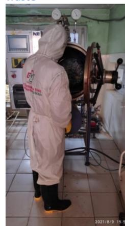
**Figure 31. Loading the bio-hazard drum in pre-vacuum autoclave for disinfection**
