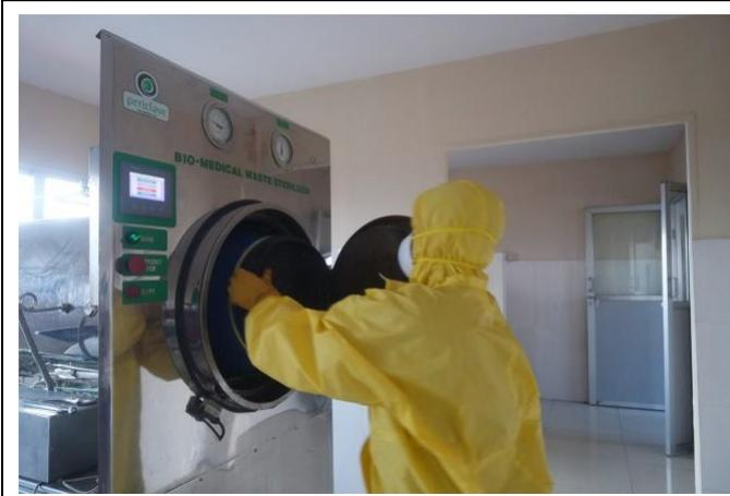
**Photo E.13.1.** Loading a bio hazard container into a pre vacuum autoclave
