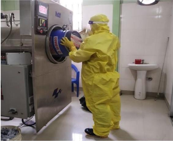
**Photo E.11.1.** Loading bio hazard containers to a pre vacuum autoclave at a hospital waste treatment facility
