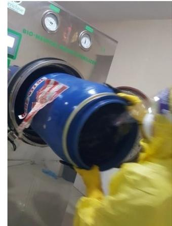
**Photo E.13.2.** Unloading a bio hazard container from the autoclave
