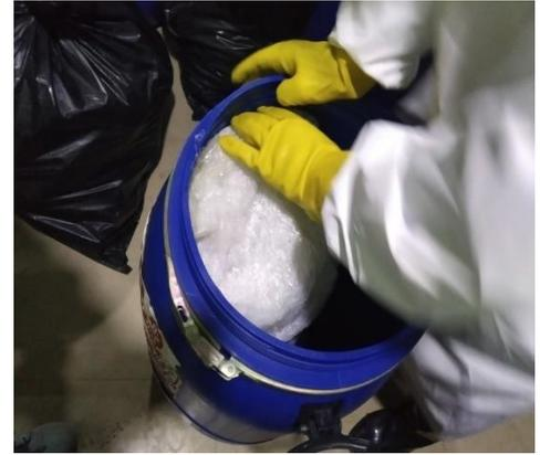
**Photo E.11.2.** Unloading a bio hazard container from the autoclave
