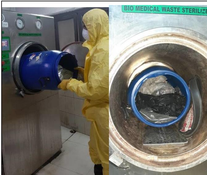
**Photo E.12.1.** Loading a bio hazard container into the pre vacuum autoclave
